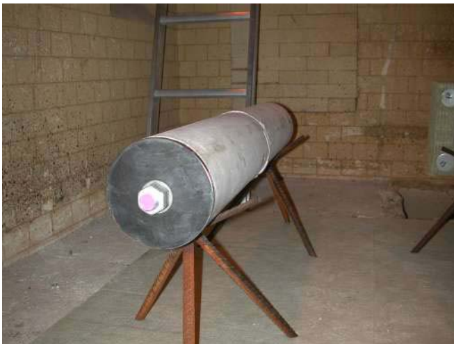
Figure E2. Unloaded cylindrical specimen placed in the furnace.
