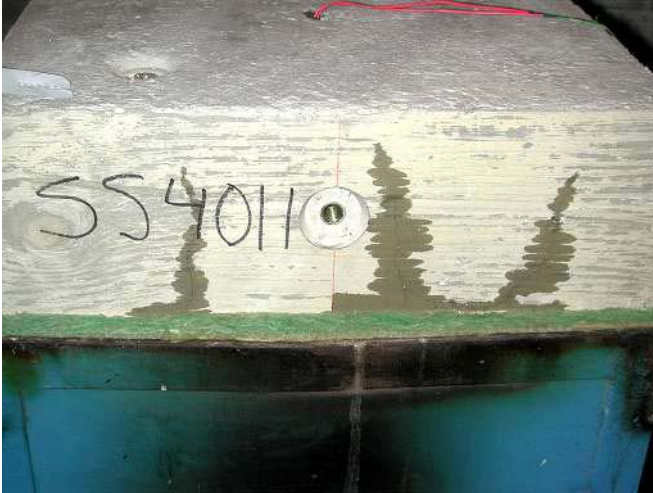
Figure E27. Small slab SS 40 11 during the fire test. Water is pouring out at the edges.
