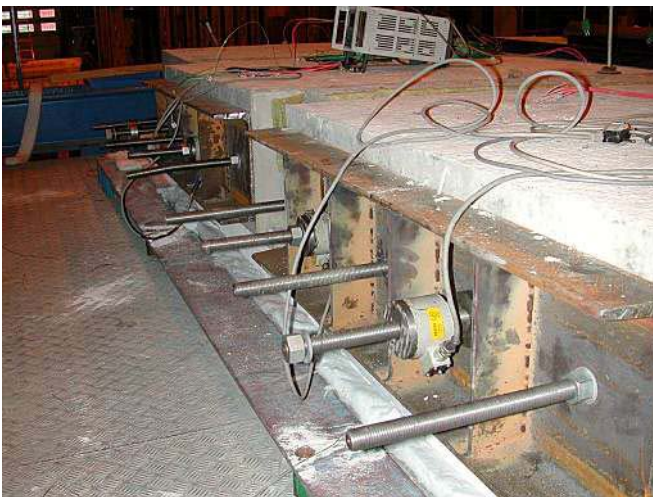
Figure F5. Stiffened steel beam for transferring load to the specimen.
