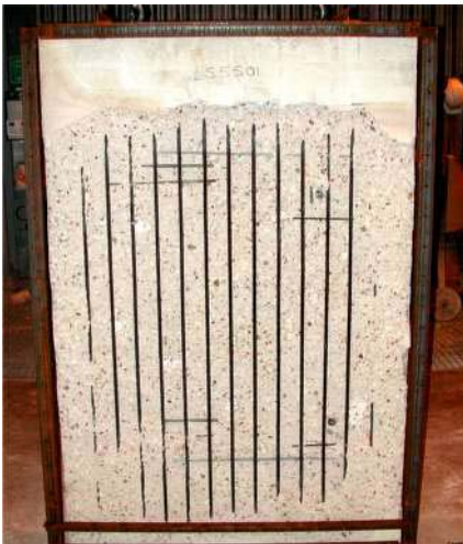
Figure D13. Slab LS 55 01 after the fire test.
