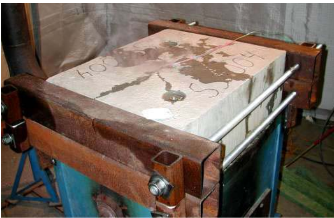
Figure E24. Small slab SS 40 04 during the fire test. Water is pouring out on the top and at the edges.
