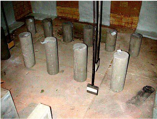
Figure F10. Cylinders on the floor of the furnace.
