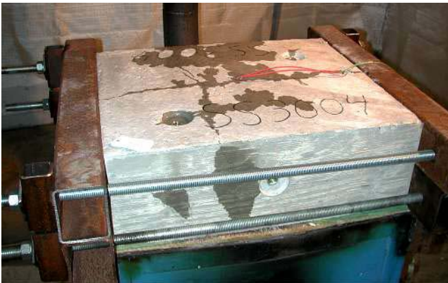
Figure E16. Small slab SS 30 04 during the fire test. Water is pouring out on the top and at the edges.
