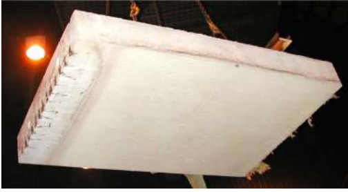
Figure D11. Slab LS 40 11 after the fire test.
