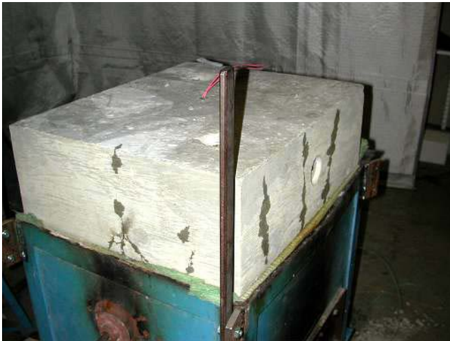
Figure E13. Small slab SS 30 02 during the fire test. Water is pouring out at the edges.
