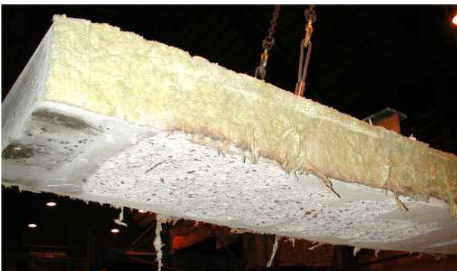
Figure D13. Slab LS 55 01 after the fire test.
