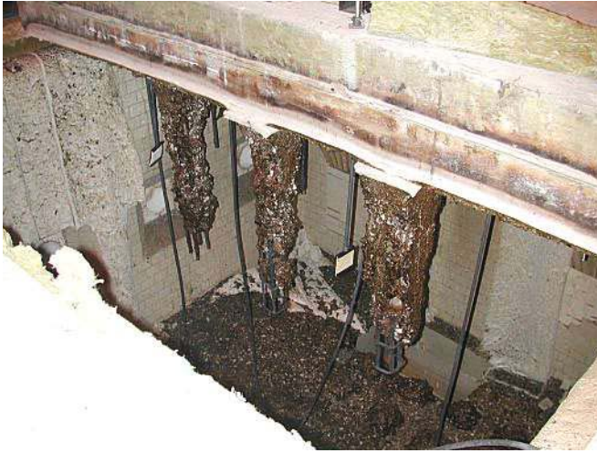
Figure F113. Columns after the first fire test. From the left: A10, C10, D10.
