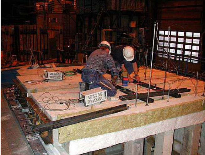
Figure F6. Mounting of specimens on the furnace.
