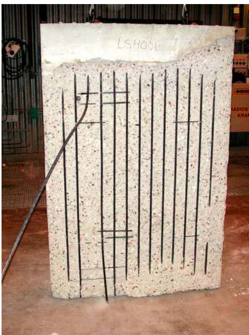
Figure D10. Slab LS 40 01 after the fire test.
