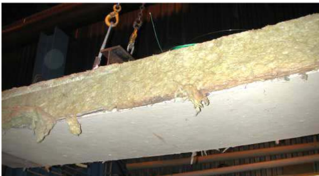
Figure D17. Beam LB 40 11 after the fire test.
