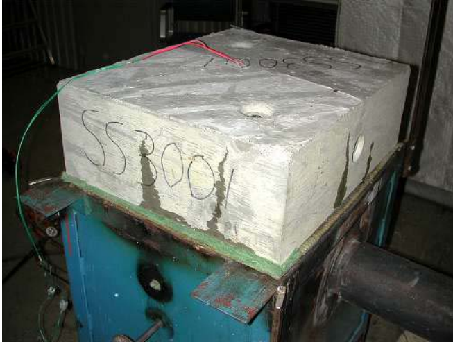
Figure E11. Small slab SS 30 01 during the fire test. Water is pouring out at the edges.
