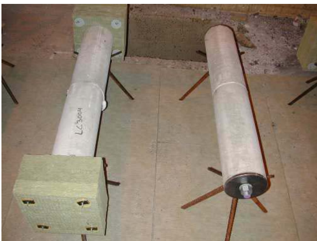
Figure E3. Loaded (left) and unloaded (right) cylindrical specimens placed in the furnace.
